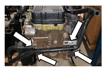
Note: Ensure that the coolant hose does not rub on the coolant tube bracket. The bracket can be angled slightly and insulated clamp can manipulated to gain clearance.
