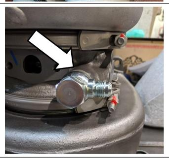
Loosely install the coolant line (1407023) as shown.
