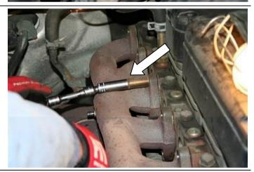
Remove the turbo/manifold as an assembly.
