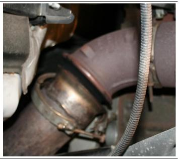
Remove the turbo oil drain with a 10mm socket and pull the line out of the engine block
