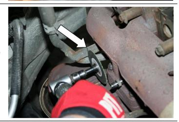
Remove the turbo oil feed from the turbo
