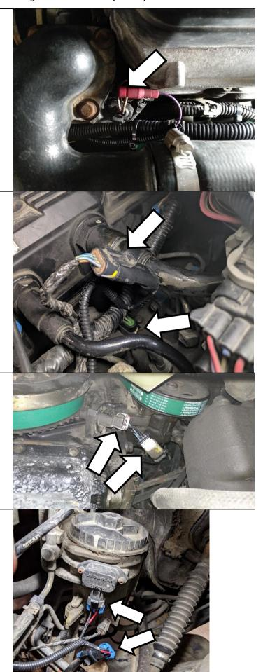
Choose the appropriate accelerator pedal position sensor adapter harness (1407130/31/32) for your model. Install this in line with the sensor.
