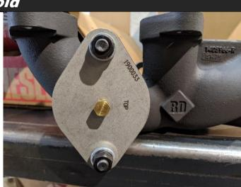
Install 2 of the longer studs in the engine as shown at the bottom of 2<sup>nd</sup> and 3<sup>rd</sup> port from the back of the motor.
