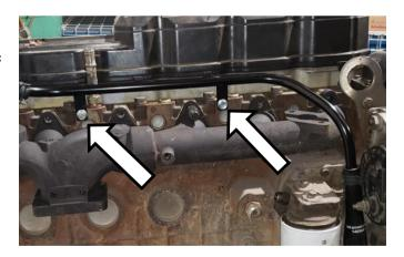
Install the (1405446) hose section onto the new coolant tube, heater core outlet and the transmission heat exchanger secting with 3 of the (1302198) spring clamps.
