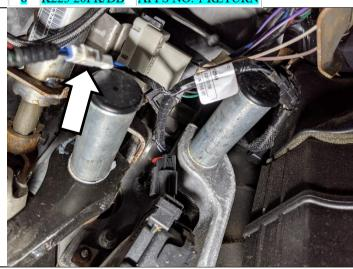
Route the RED and PINK wires from the toggle switch kit (1407038) from inside the cab to under the hood near the VGT control module.
