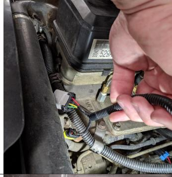
Connect the turbocharger actuator and the turbocharger speed sensor wires to the turbo.
