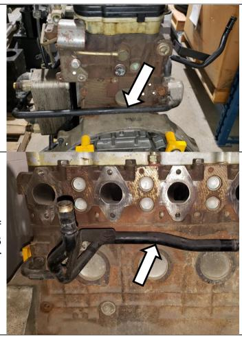
Finally remove the front section which connects to the water outlet fitting and then remove the water outlet fitting.
