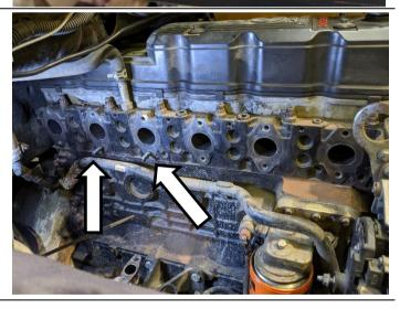
Remove the coolant port plug, towards the front of the engine on the passenger side.
