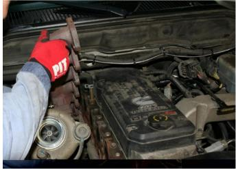
Special Note: Install Supplement Kit 1047137 which is for 2003-2005 automatic transmission models. This kit relocates the coolant pipes from the heater core/transmission cooler and water inlet connection from below the exhaust manifold to above. (Not required on trucks without a transmission oil cooler or when a coolant bypass kit has been installed)
