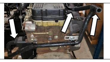
Mount the (1407034) coolant tube bracket (supplied from the Howler Install Kit) to the lower exhaust stud of the #6 cylinder reusing the OE M10 flange nut.
