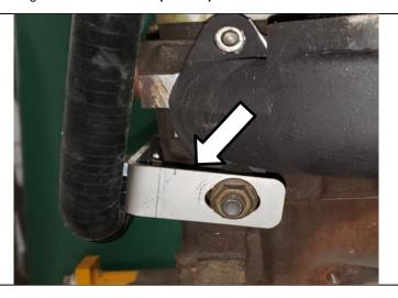
Install the 2 insulated clamps (1120125) around the coolant hose section that goes behind the engibe block. Secure passenger side clamp by mounting to the coolant tube bracket with 1 of the
