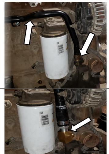
Install the 90deg fitting (FT-69884) into the water inlet housing port and orientate to face upward.
