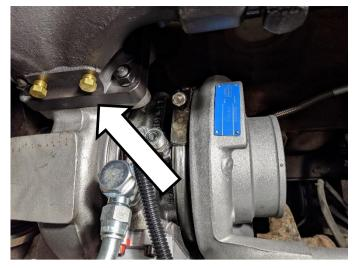
Secure the coolant tube to the manifold using the provided bracket.
