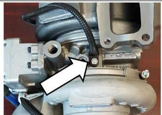
Loosely install the Banjo to JIC fittings in the bottom of the turbocharger.
