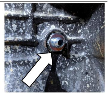
Install the speed sensor (1407043) into the turbocharger.
