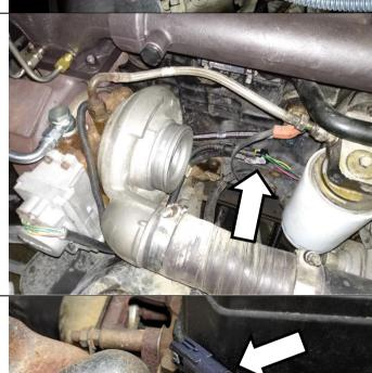
2004-2007 Models Connect the main harness to the coolant temperature sensor by plugging it inline.
