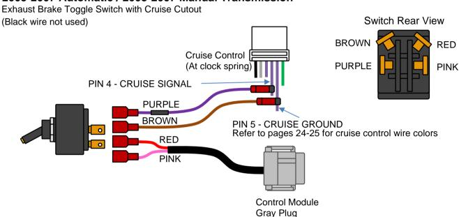
**NOTE** The light in the toggle switch will be on whenever the ignition is on. If you prefer the light to be on only when the brake is turned on, then reverse the RED and PINK wires at the toggle switch.
